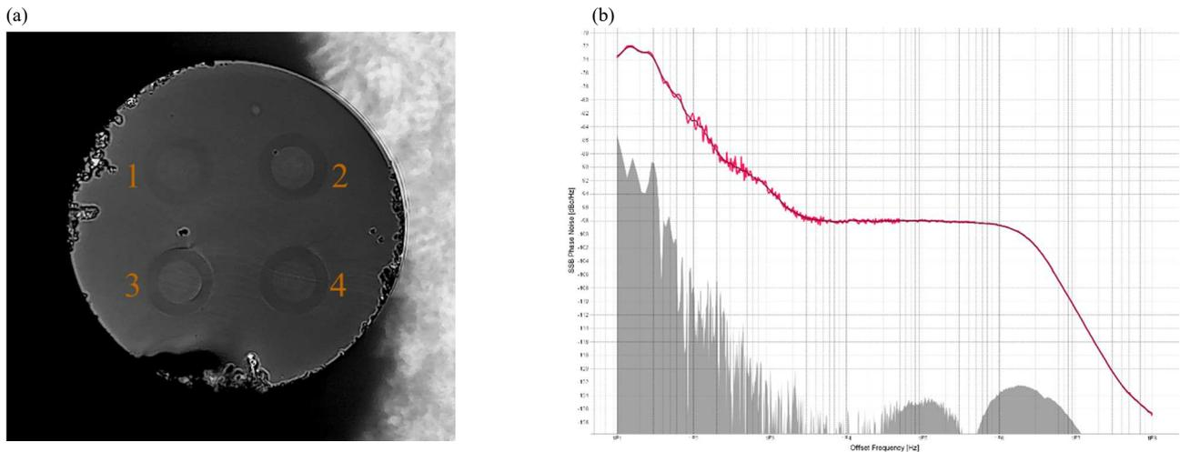
Fig. 2. a) The cross section of 4-core fiber. Cladding diameter:  $125 \mu\text{m}$ . b) Phase noise of transmission stability of 1 GHz radio frequency signal in 3 km MCF link.
