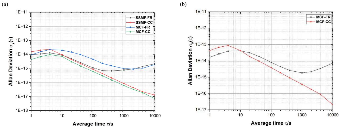
Fig. 3. Allan deviation of transmission stability of 1 GHz frequency signal in 3 km link (a) and 6 km link (b). FR: free running, PID function is not turned on, CC: closed-loop control, PID function is turned on.
