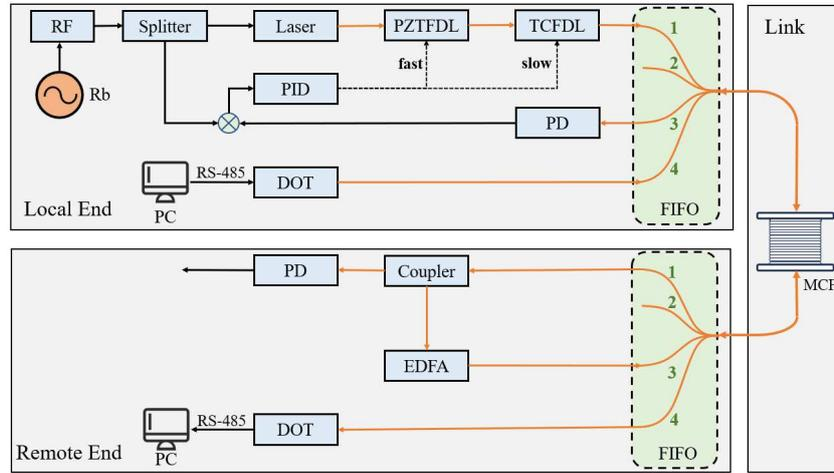
Fig. 1. Schematic of the radio frequency transmission system based on 4-core fiber. Rb: Rubidium clock, RF: radio frequency, PZTFDL: piezoelectric ceramics fiber delay line, TCFDL: temperature control fiber delay line, FIFO: fan-in-fan-out, MCF: multi-core fiber, PD: photodetector, EDFA: Erbium-doped fiber amplifier, PID: proportion integration differentiation control, PC: Personal Computer, DOT: Digital optical transmission module.
