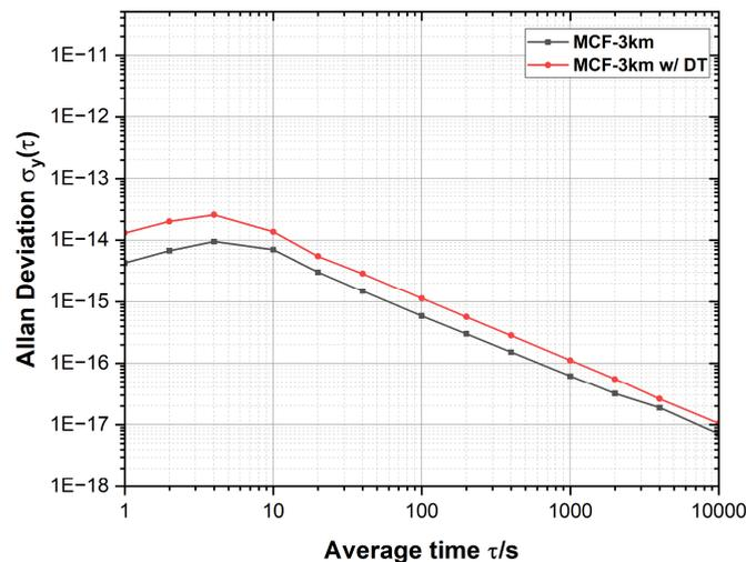
Fig. 4. Allan deviation of transmission stability of 1 GHz frequency signal with or without data signal transmission in 3 km link. DT: data signal transmission.
