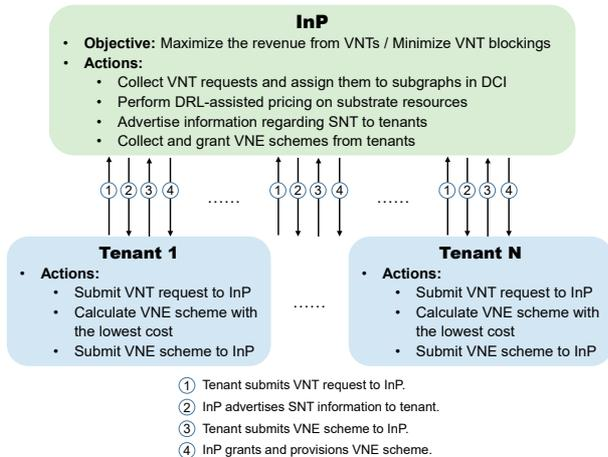
Fig. 1. Service framework for distributed and tenant-driven VNT slicing.
