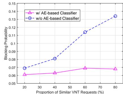
Fig. 11. Performance comparison of DRL-GRC-VNE with and without AE-based classifier (56 SNs in 4 subgraphs, and traffic load at 300 Erlangs).
