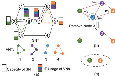
Fig. 6. Example on solving VNE selection, (a) SNT, VNTs and VNE schemes, (b) building CG for VNE schemes, and (c) finding MWIS in CG.
