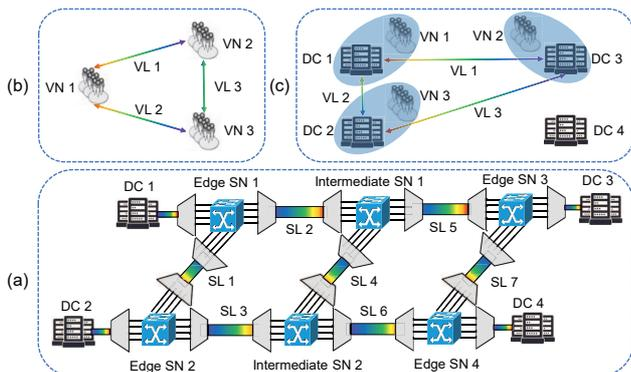
Fig. 3. Example on VNT slicing in a subgraph of DCI, (a) the SNT, (b) a tenant's VNT request, and (c) the VNE scheme computed by the tenant.
