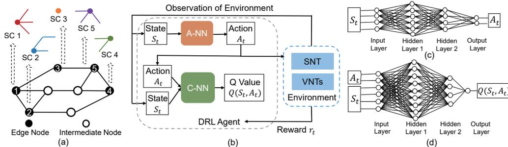
Fig. 4. (a) Example on partitioning an SNT into SCs, (b) DDPG-based DRL model for resource pricing and advertising, and (c) and (d) Architectures of A-NN and C-NN, respectively.
