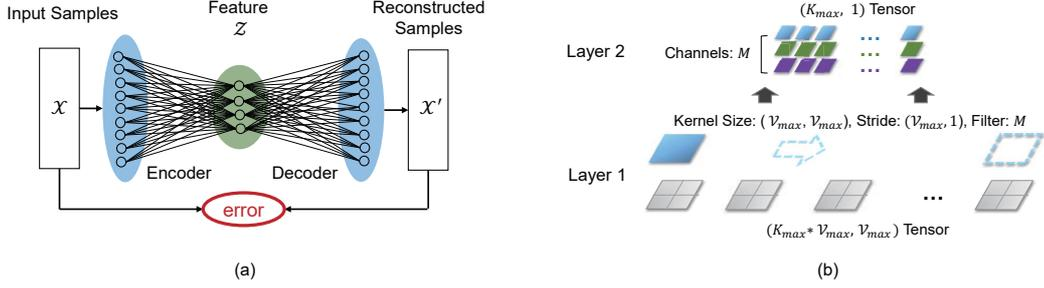
Fig. 5. (a) Generic principle of AE, and (b) AE-based VNT compression.
