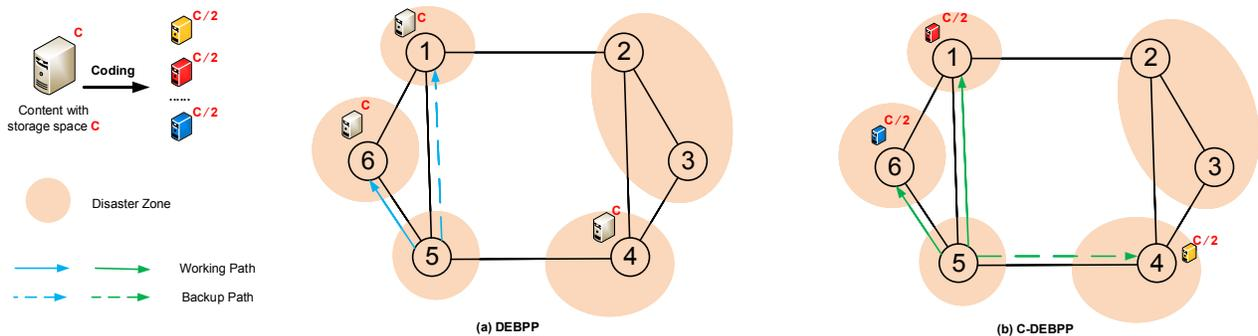
Fig. 1. Solution acquired by DEBPP and C-DEBPP with 6-node topology and 5 DZs.
