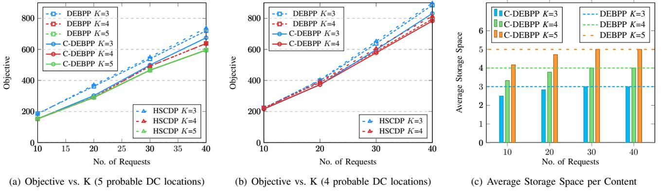
Fig. 2. System Performance for different No. of probable DC locations in NSFNET.
