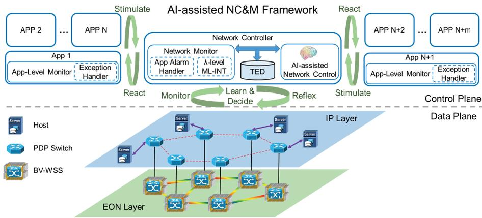
Fig. 2. Our AI-assisted NC&M framework, APP: application, TED: traffic engineering database (adapted from [18]).
