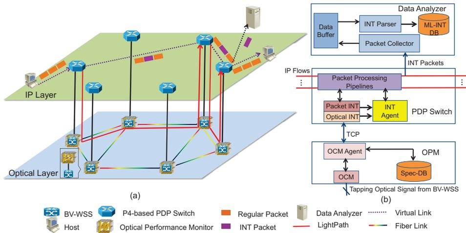
Fig. 1. System architecture of our flexible ML-INT system, ML-INT DB: multilayer INT database, Spec-DB: optical spectrum database (adapted from [22]).
