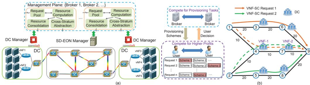
Fig. 1. (a) Network architecture of an EO-IDCN and (b) an example for profit-driven VNF-SC provisioning.
