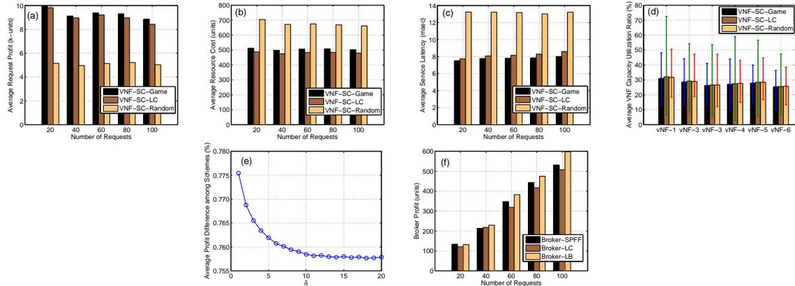
Fig. 2. Simulation results on (a) average request profit, (b) average resource cost, (c) average service latency, (d) average VNF capacity utilization ratio, (e) average profit difference among schemes within a request and (f) broker profit.
