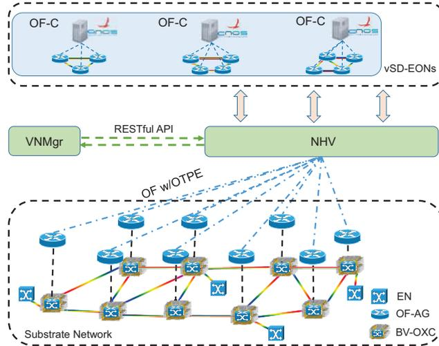
Fig. 1. Architecture of our QoS-aware survivable vSD-EON slicing system, OF-C: ONOS-based OpenFlow controller, VNMgr: Virtual network manager, NHV: Network hypervisor, RESTful API: RESTful application programming interface, OF w/ OTPE: OpenFlow with optical transport protocol extensions, EN: End-node, OF-AG: OpenFlow agent, BV-OXC: Bandwidth-variable optical cross-connect.
