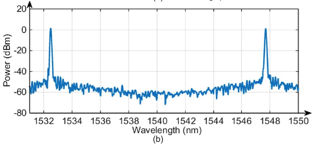
Fig. 8. Experimental results for lightpath activation, (a) Wireshark capture of messages used, and (b) spectra of the established lightpaths in two vSD-EONs.
