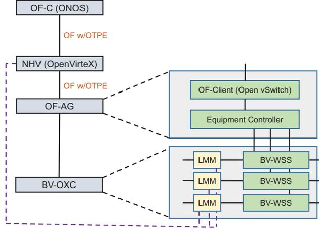
Fig. 2. Zoom-in view of the vertical structure of a vSD-EON, OF Client: OpenFlow client, BV-WSS: Bandwidth-variable wavelength-selective switch, LMM: Link monitoring module.
