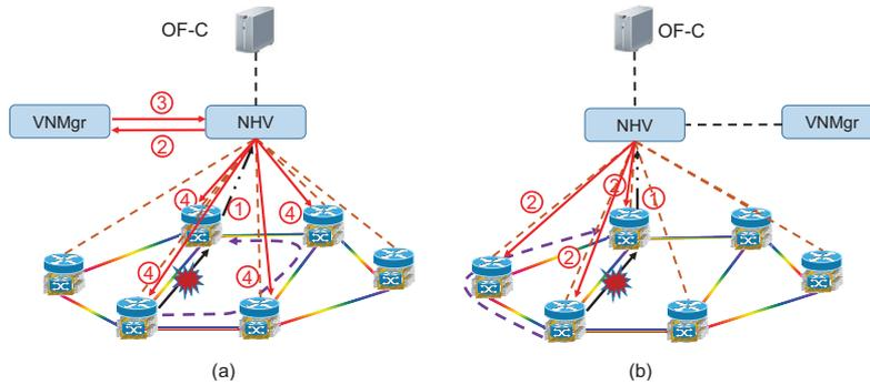
Fig. 4. Transparent DP restoration schemes for vSD-EONs using (a) on-demand VL remapping, and (b) "1:1" VL protection.
