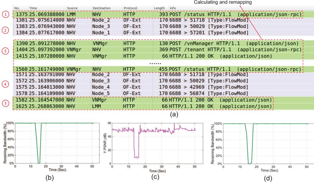
Fig. 9. Experimental results for DP restorations, (a) Wireshark capture of messages used, (b) receiving bandwidth of video streaming in *Tenant 1*, (c) Y-PSNR of video playback in *Tenant 1*, and (d) receiving bandwidth of bulk file transfer in *Tenant 2*.
