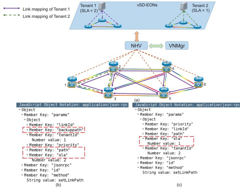
Fig. 6. Experiments of vSD-EONs creation, (a) substrate topology, and the control messages from VNMgr to NHV for embedding (b) a VL with "1:1" VL protection and (c) a VL with on-demand VL remapping.
