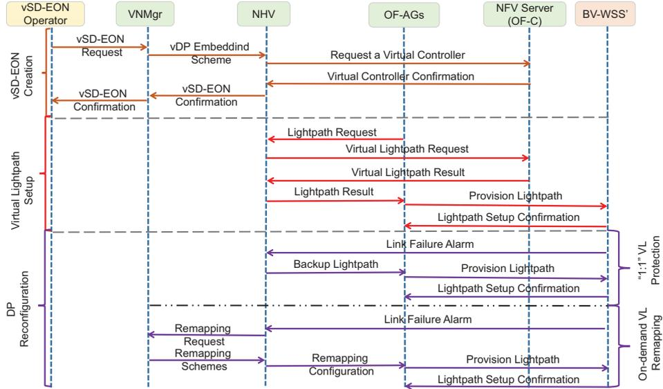
Fig. 3. Operation procedure for vSD-EON creation, lightpath establishment, and transparent DP restoration.
