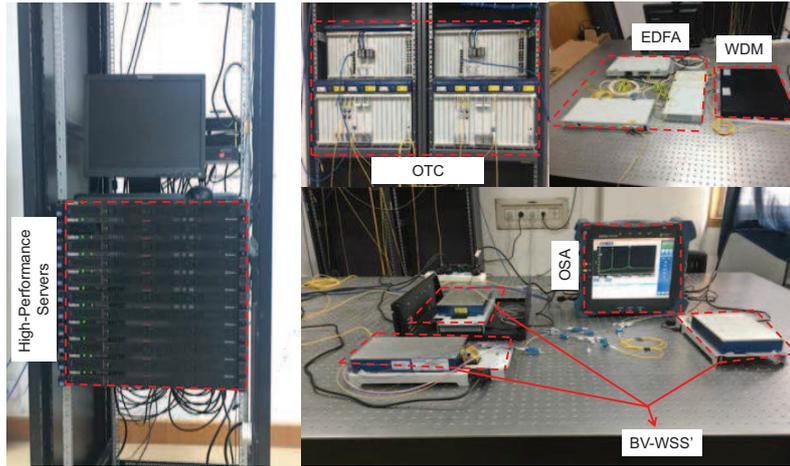
Fig. 5. Experimental testbed, OTC: Optical transmission chassis, OSA: Optical spectrum analyzer, EDFA: Erbium-doped optical fiber amplifier, WDM: Wavelength-division multiplexer/demultiplexer.
