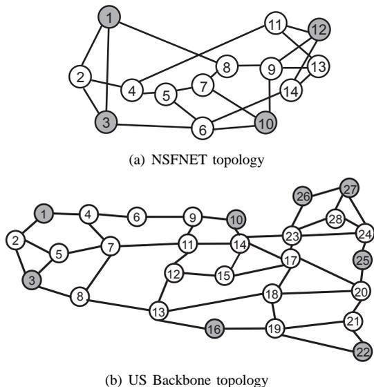
Fig. 2. Domain topologies with border nodes marked as grey.
