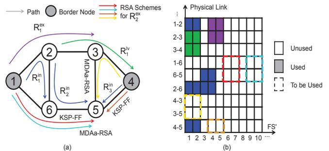
Fig. 1. Example on lightpath provisioning in a domain of MD-EON
