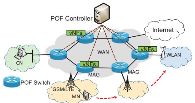
Fig. 3. Architecture of a POF-based mobile network.
