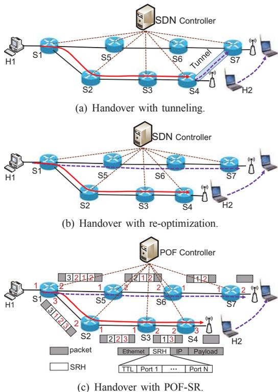
Fig. 2. Handover schemes in SDN-based mobile networks.
