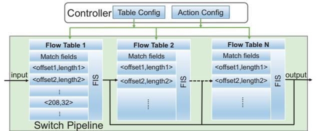
Fig. 1. Packet forwarding procedure in POF.
