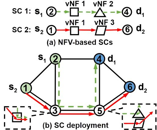
Fig. 1. SC deployment with vNF placement and link mapping.
