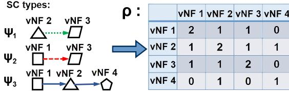
Fig. 4. Example on quantifying the affiliation of vNFs with  $\rho_{m,m'}$ .
