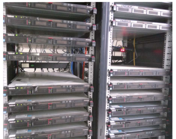
Fig. 5. SD-EON control-plane testbed built with Linux servers.
