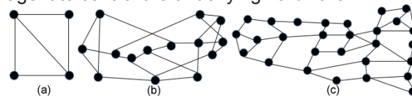
Fig. 2: (a) 4-node mesh network; (b) 14-node NSFNET; (c) 24-node US Backbone
