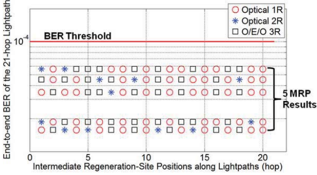
Fig. 4. MRP results for a 21-hop lightpath obtained by the GA.
