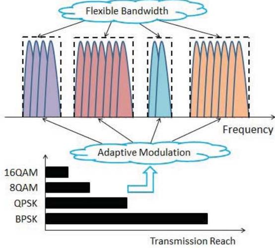
Fig. 1. Elastic bandwidth allocation in O-OFDM systems.
