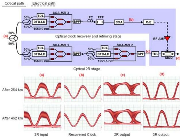
**Fig. 3: All-optical 3R regenerator setup, TDL: Tunable delay line; DFB-LD: DFB laser diode; SOA-MZI: Semiconductor optical amplifier based Mach-Zehnder interferometer; BPF: Optical band-pass filter; PC: Polarization controller; FPF: Fabry-Perot filter; SOA: Semiconductor optical amplifier; O/E: Optical-to-electrical converter; RF AMP: RF amplifier; MOD: LiNbO<sub>3</sub> modulator**
