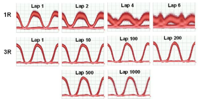
**Fig. 4: Eye-diagrams of 264 km fiber recirculation loop experiments**
