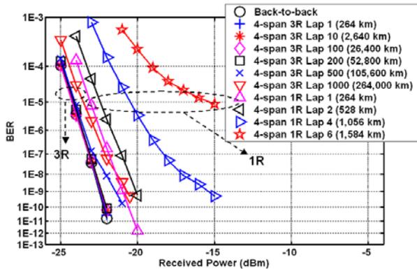
Fig. 5: BER measurement results of 264 km fiber recirculation loop experiments
