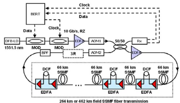
**Fig. 2: Experimental setup, BERT: Bit-error-rate-tester, DFB-LD: DFB laser diode; MOD: LiNbO<sub>3</sub> modulator; AOM: Acoustic optical modulator; BPF: Optical band-pass filter; EDFA: Erbium-doped fiber amplifier; SSMF: Standard single-mode fiber; DCF: Dispersion compensating fiber; RX: Optical receiver**
