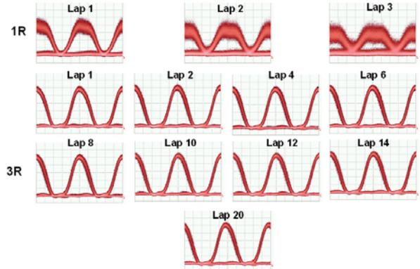
Fig. 6: Eye-diagrams of 462 km fiber recirculation loop experiments
