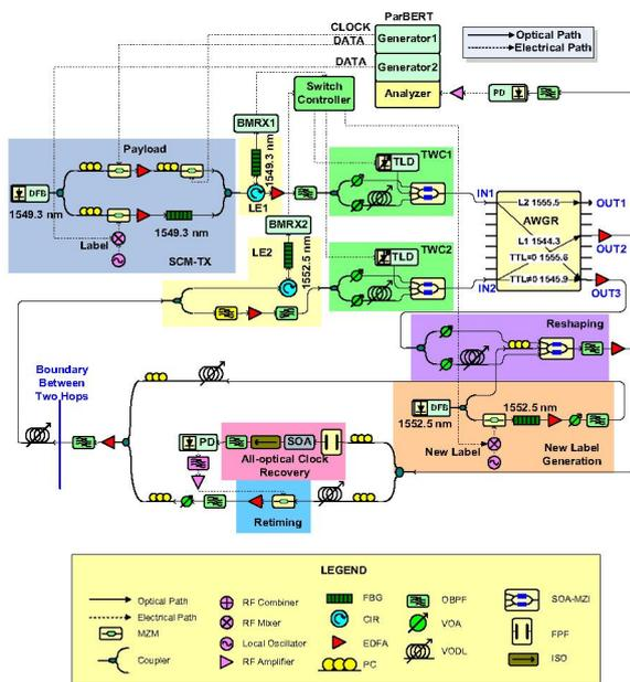
Figure 3: Simplified experimental setup. The text in the AWGR indicates the condition and the wavelength in nm for the switching.
