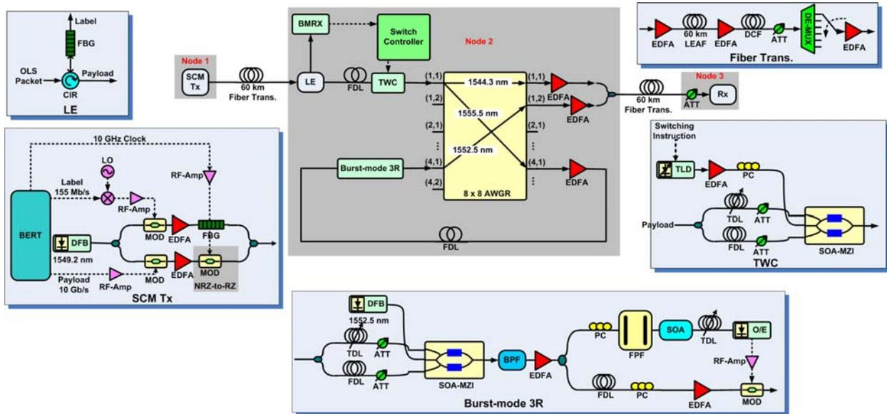
Fig. 2 Experimental Setup, BERT: Bit-error-tester, LO: Local oscillator, RF-amp: RF amplifier, EDFA: Erbium-doped fiber amplifier, CIR: Optical circulator, BMRX: Label burst-mode receiver, DE-MUX: De-multplexer, PC: Polarization controller, TDL: Tunable delay line, FDL: Fixed delay line, BPF: Band-pass filter, O/E: Optical-to-electrical converter, Rx: optical receiver.
