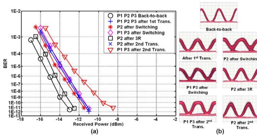
Fig. 4 Experimental results, (a) BER curves, (b) Eye-diagrams.
