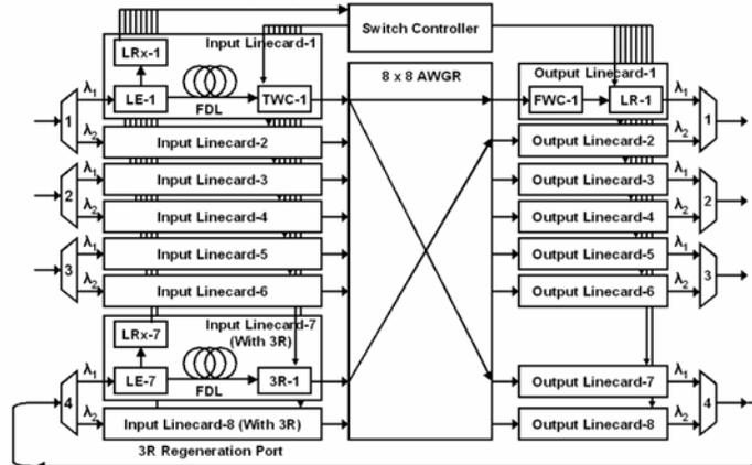
Fig. 1 Simplified architecture of an OLS router with limited 3R capability, LE: label extractor, LRx: label receiver, TWC: tunable wavelength converter, AWGR: arrayed waveguide grating router, FWC: fixed wavelength converter, LR: label rewriter.
