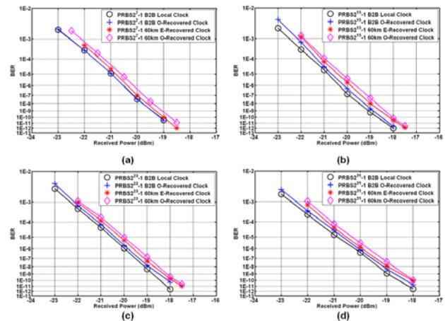
**Fig 3 BER measurement results for back-to-back and after 60 km transmission, when the signal is encoded with (a) PRBS  $2^7-1$ , (b) PRBS  $2^{15}-1$ , (c) PRBS  $2^{23}-1$ , and (d) PRBS  $2^{31}-1$**
