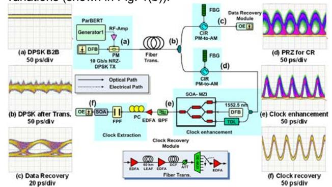
**Fig. 1 Experimental Setup, ParBERT: Parallel Bit-Error-Rate Tester, ATT: optical attenuator, BPF: optical band-pass filter, CIR: optical circulator, DFB: DFB laser diode, TDL: tunable delay line, OE: Optical to Electrical Converter, PM: phase modulator, PM-to-AM: phase modulation to amplitude modulation conversion, DEMUX: optical wavelength demultiplexer, (a)-(e) Eye diagrams measured at different locations as labeled in the setup**
